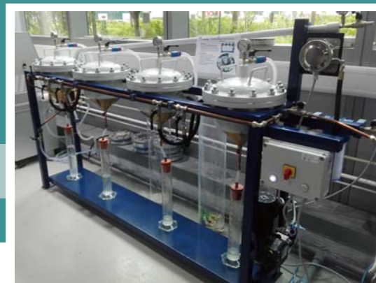
Automatic concrete water permeability apparatus (CRD-C 48-92)
